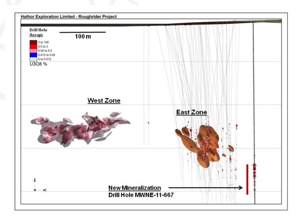
Figure 3. A cross-sectional view of a three-dimensional block model of the Roughrider system, view north. Outline of West Zone is from recent NI43-101 report (Keller et al. 2011). The grade shell (1%  $U_3O_8$ ) for East Zone was produced using Leapfrog 3D geological modelling software. The new mineralization in Hole 11-667 is 100 m east of the core of East Zone, and deeper. Horizontal = vertical scale.
