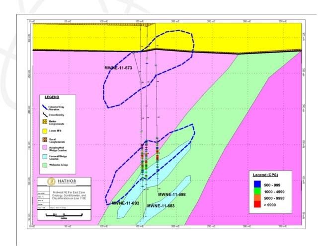
Figure 3. Cross Section, Far East Zone, Roughrider Project, Line 110E, view easterly.
